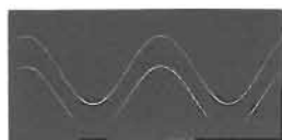
SCALE: X = 0.2 ms/DIV Y = 2.0 V/DIV V_{DD} = V_C = +7.5V, V_{SS} = -7.5V, R_L = 10K\Omega C_L = 15 pF f_{IG} = 1 kHz, V_{IG} = 5V p-p DISTORTION = 0.2%
