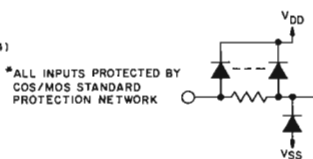
Fig. 1 - Schematic Diagram - Input circuit and 1 of 6 identical inverter/buffers.
